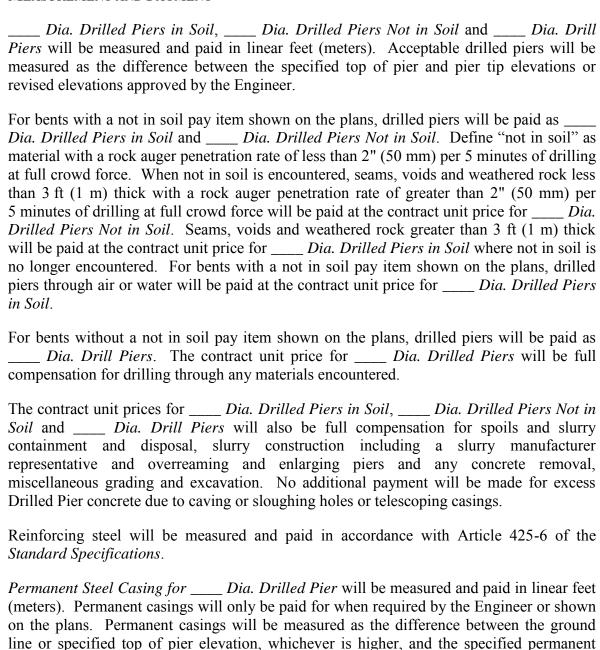
casing tip elevation or revised elevation approved by the Engineer. If a permanent casing cannot be installed to the tip elevation shown on the plans, up to 3 ft (1 m) of casing cut-off
